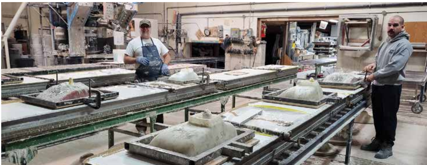
Mike Bedard and Sam Deverell working on casting vanity tops.
