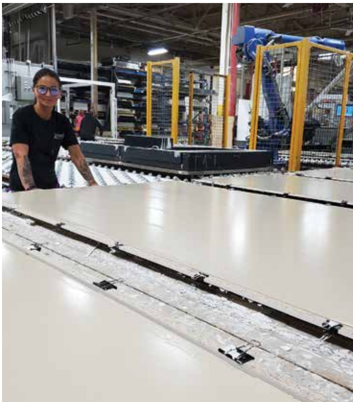
Solid Surface Team Leader Shannon Goodyear getting ready to demold a shower panel that was just cast.
