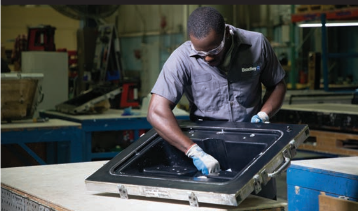
A plant employee works on making a mold of the natural quartz surface.
