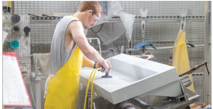
Wet polishing is performed on a natural quartz surface.
