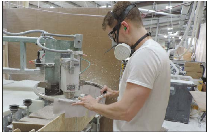
A grinding machine helps to shape a custom shower caddy.
