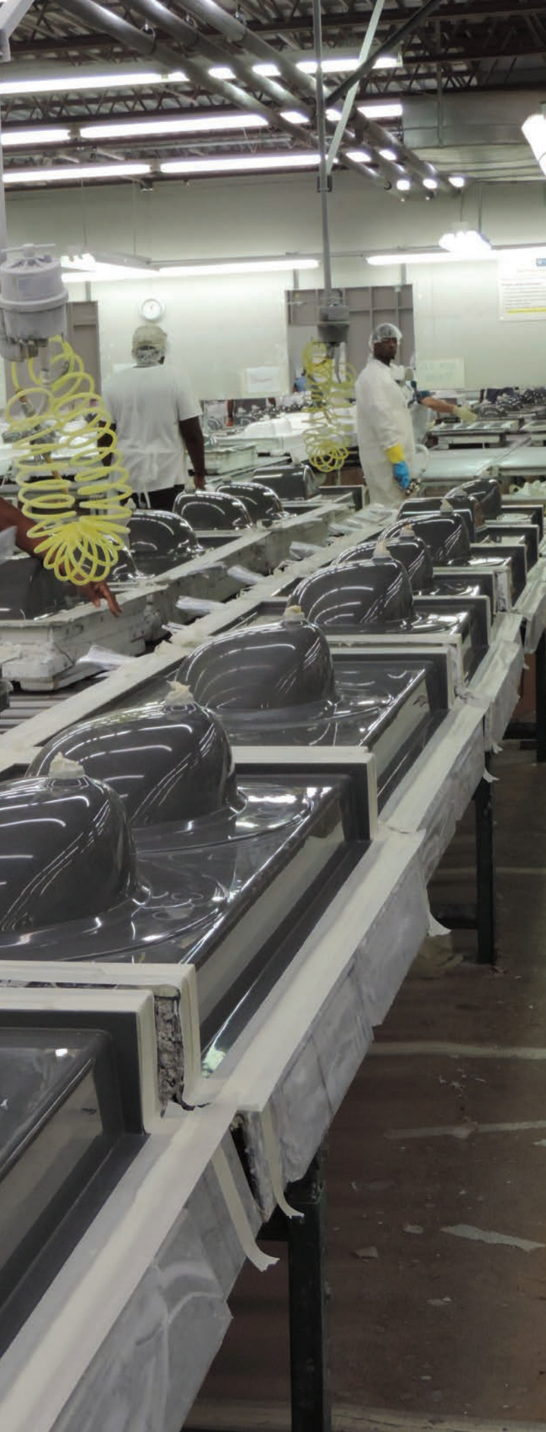
Molds are prepared in one of two Virginia Marble cast polymer manufacturing plants.
