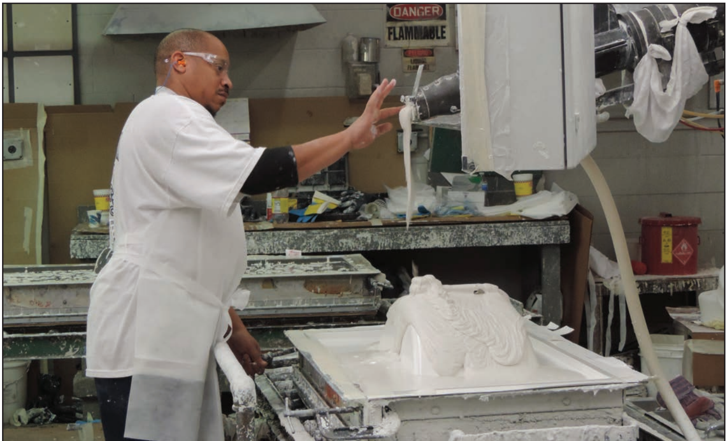
Group leader Jacoby Freeman casts directly onto a Wave Bowl mold at the company's Brunswick Avenue plant.
