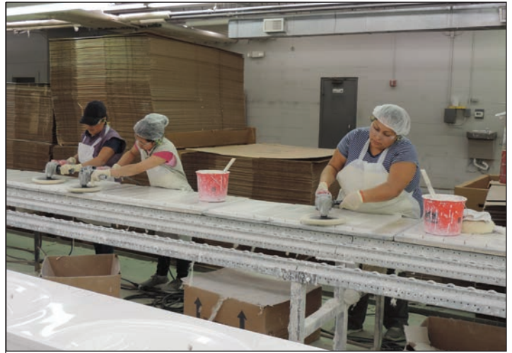
Workers on the line polish and finish end splashes.
