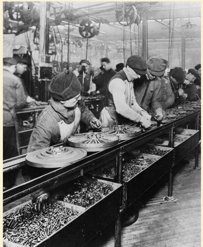
Ford assembly line, 1913. The magneto assembly line was the first of its kind.
