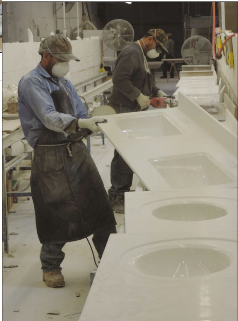
Employees give sinks the final touch on the marble finishing line.
